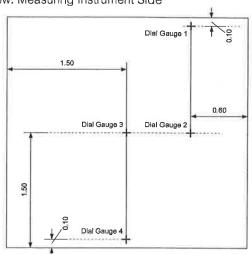
Permanent Deformation Observed in millimeters.
